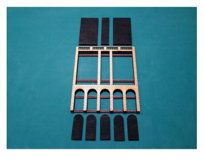
Looking from the front-side (engraved side) of the frame, the "window" inserts are laid out in their relative positions. The inserts are not specific to any wall, and any piece of the correct shape can be used anywhere.
