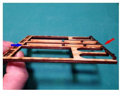
Glue the two spacers to the back-side of the frame. The #1 notch on the spacer rests on top of the grooves in rib F1 (red arrow). Center the spacer down the middle of the spine on the frame (blue arrow). See the arrows in the next image for another view.
