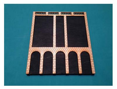
Lay the inserts into the openings and glue to the ribs behind. Be sure the inserts are pressed all the way down. If you were careful when attaching the ribs to the back-side the inserts should slide in easily.
