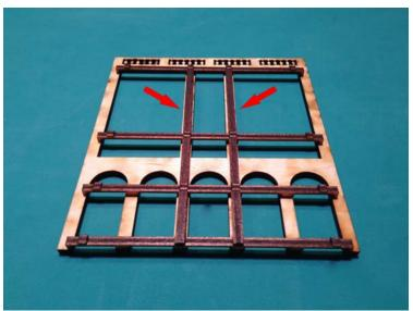
Glue the F2, F3, and F4 ribs to the back-side of the frame using the notches in the spacers to position them. As with rib F1 previously, the numbered side of these ribs face to the bottom.
